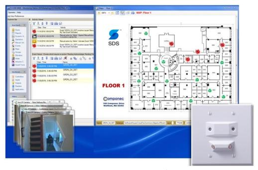
The SDS/C-CURE 9000 Connector displays shot locations on a floor plan map and populate alarms within the C-CURE alarm interface. Cameras can be configured to pull live video of the event to the forefront. Inset: SDS gunshot sensor.
